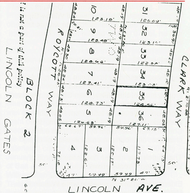
Lot Plan of east end of Lincoln Gates, Block 2. Lots are numbered around the block, beginning at the corner of Lincoln and Clark and ending with Lot No. 36 on Clark.
